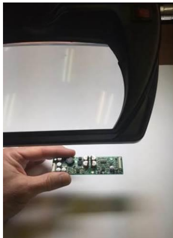
Single shadow from wide-angle, diffused LEDs, similar to fluorescent source
