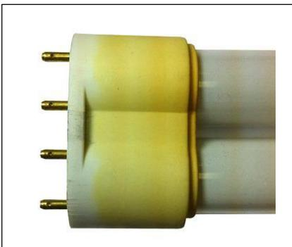
Discoloration of plastic base due to UV emitted from 36-Watt 4-pin CFL Fluorescent Bulb
